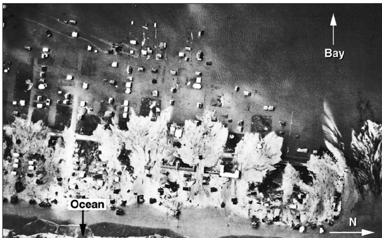
Figure 3-6. Flooding, erosion, and overwash at Fenwick Island, DE, following March 1962 nor'easter
